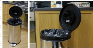
Figure 2. A BinCam bin augmented with a Sony Ericson Xperia™ X10 mini smart phone.
